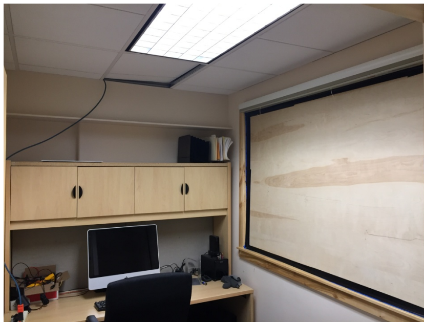
Figure 1. LED testing room at the RTF. The plywood is covering the interior window; it was taped in place to block all light infiltration.
