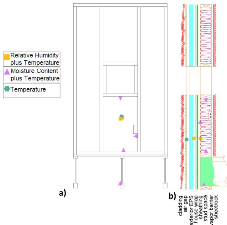
**Figure 1.** (a) An elevation view of the basic construction of each wall and (b) a cross section of wall 3. All nine walls had similar construction and the same sensor layout.
