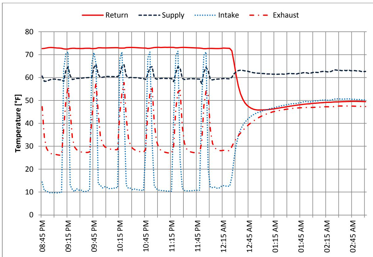
Figure 18. Freezing of the ERV core at temperature above 14 °F as a result of deactivated frost protection. Return is the return temperature from the living space, supply is the temperature supplied to the living space.
