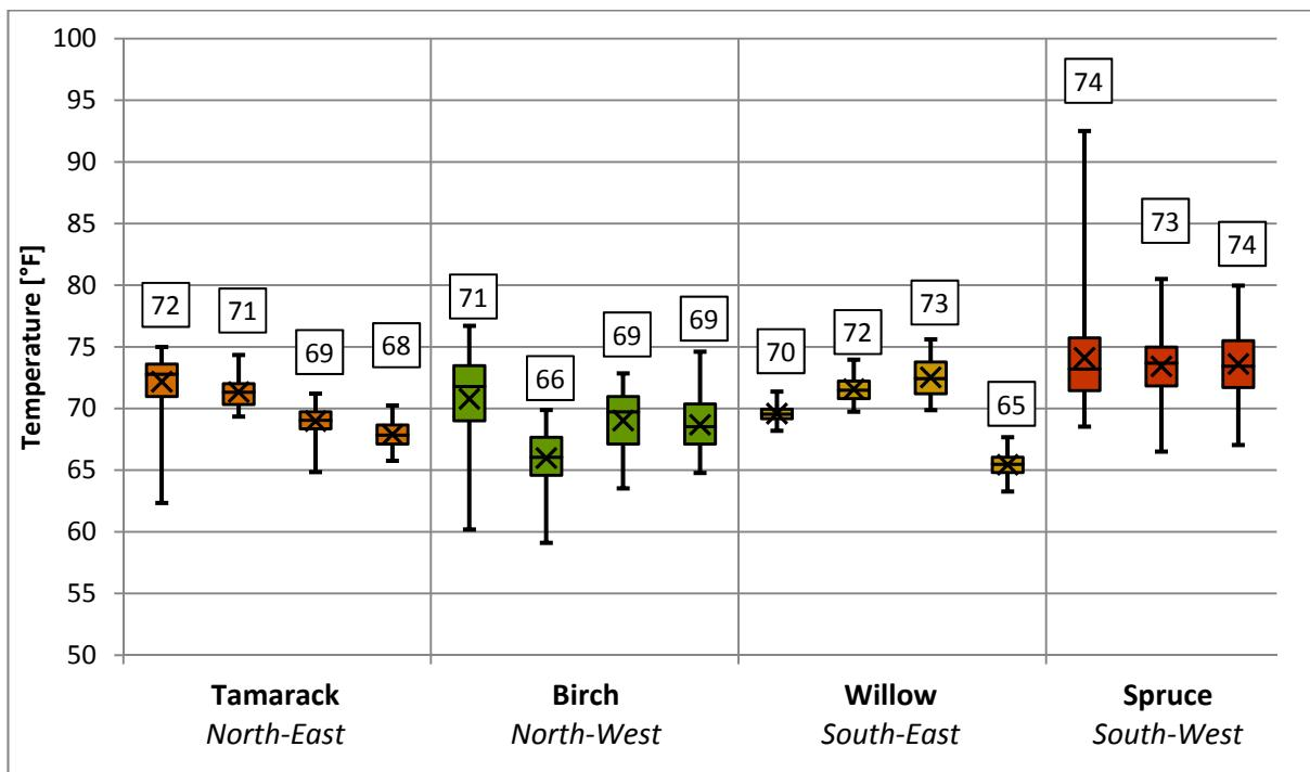
**Figure 11. Temperature distribution in bedrooms. The colored boxes describe the lower and upper quartiles, the bands inside the boxes are medians, crosses are mean values and the ends of the whiskers represent 1<sup>st</sup> and 99<sup>th</sup> percentiles.**
