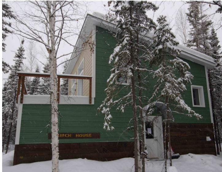
**Figure 4. Birch house.** This house has 5.5 inches (14 cm) of fiberglass batt in the stud space and 8 inches (20cm) of rigid polystyrene foam on the outside of the sheathing.
