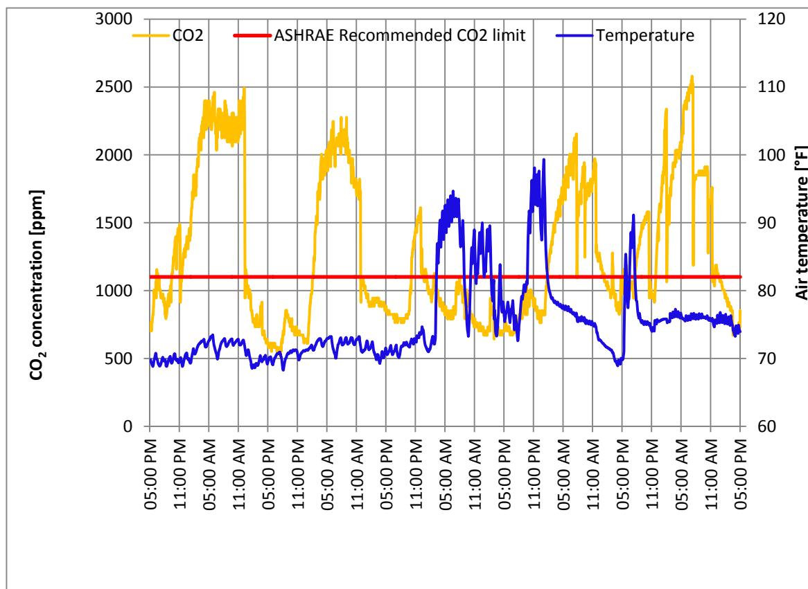
**Figure 19. Temperature and CO<sub>2</sub> concentration in a Spruce house bedroom. The bedroom is above the ASHRAE recommended 1100 ppm most of the time the room is occupied.**
