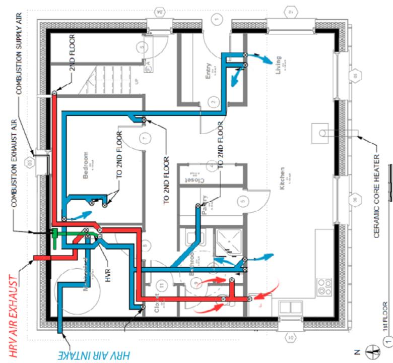
**Figure 10.** Southwest house ventilation layout. Air is supplied to the bedrooms and main living air (blue arrows). The return vents pull air from the bathroom, hall, and kitchen air (red arrows).
