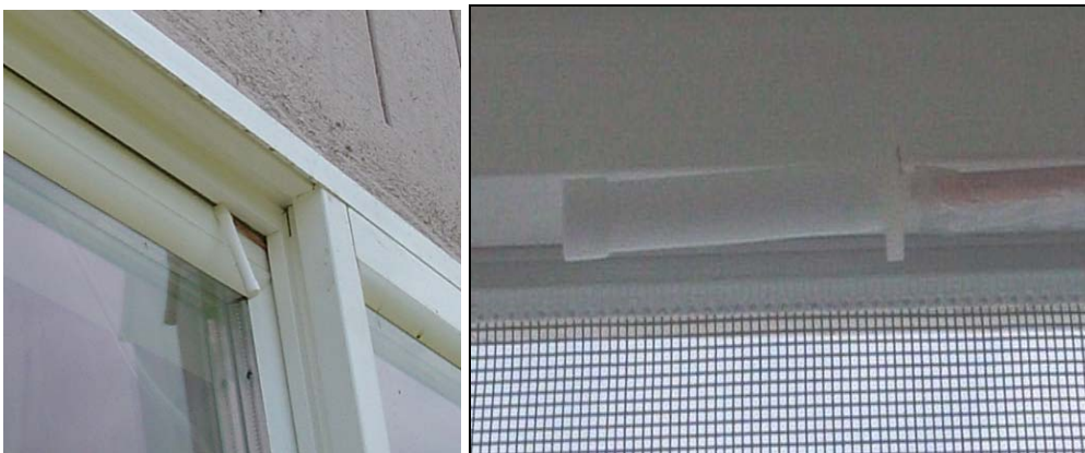
Figure 6: Outside reference pressure hose was terminated with an aquarium air bubble diffuser as a wind damper.
