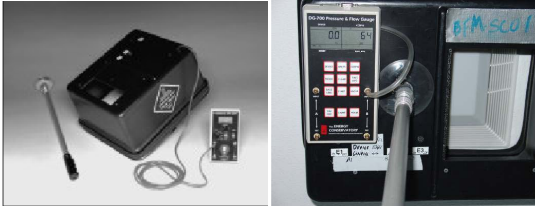
Figure 3: The Energy Conservatory's Exhaust Fan Flow Meter with DG-700 Pressure & Flow Gauge.
