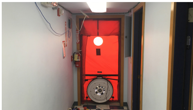
Figure 18: A blower door test helped identify air leaks for the weatherization crew to seal at the health clinic.
