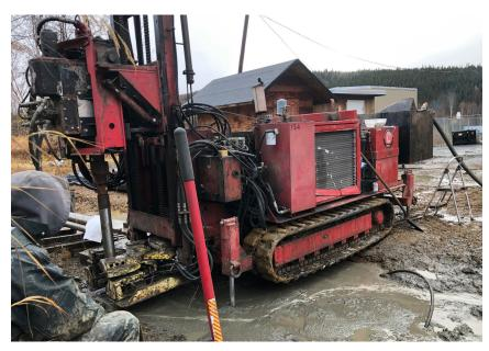
Figure 4: The drill rig used to install the ground loop coils for the ground source heat pump for the Tribal Office in Ruby, Alaska.
