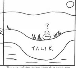
The part of the active layer that does not freeze is called a talik. It is very wet soil that remains suspended in the permafrost layer.
