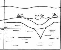
If an ice wedge is exposed, it will begin to melt. A pond will form if the active layer and ice wedge melt lower.
