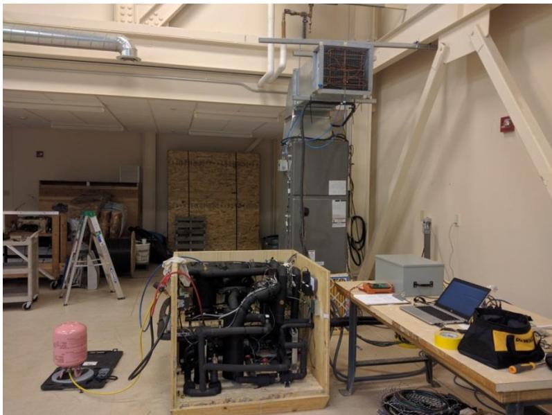
Figure 2: Indoor Unit, Compressor Compartment and Data Acquisition of Field Testing Heat Pump in Fairbanks, Alaska
