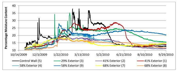
Figure 3 The moisture content of the base plate. These data are only for the first winter and summer drying season. The erratic spikes and dips in the winter for the walls 1 and 3 are due to freezing of the moisture in the stud, changing the signal of the sensor. Wall numbers are in parenthesis.
