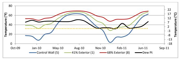
Figure 4 Average monthly temperatures on the interior surface of the sheathing plane. The three walls presented were 2x4 construction with R-11 (RSI-1.9) fiberglass batt. Wall numbers are in parenthesis.
