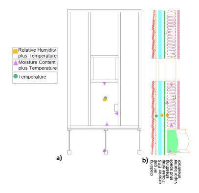
Figure 1. (a) An elevation view of the basic construction of each wall and (b) a cross section of wall 3. All nine walls had similar construction and the same sensor layout.
