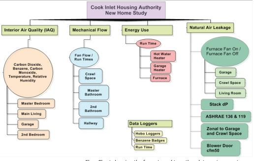
Flow Chart showing the format used to gather data on temperature, relative humidity, carbon monoxide, heating run-times, ventilation fan run-times, air quality and much more.
