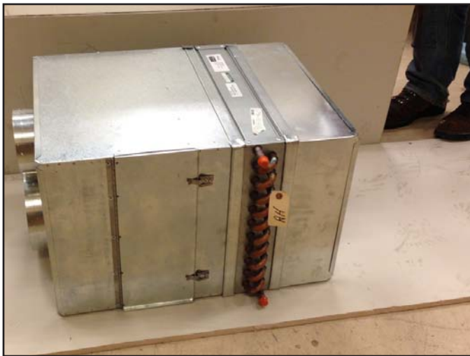
Fig 8.2 The fabricated heat exchanger mechanism before installation.
