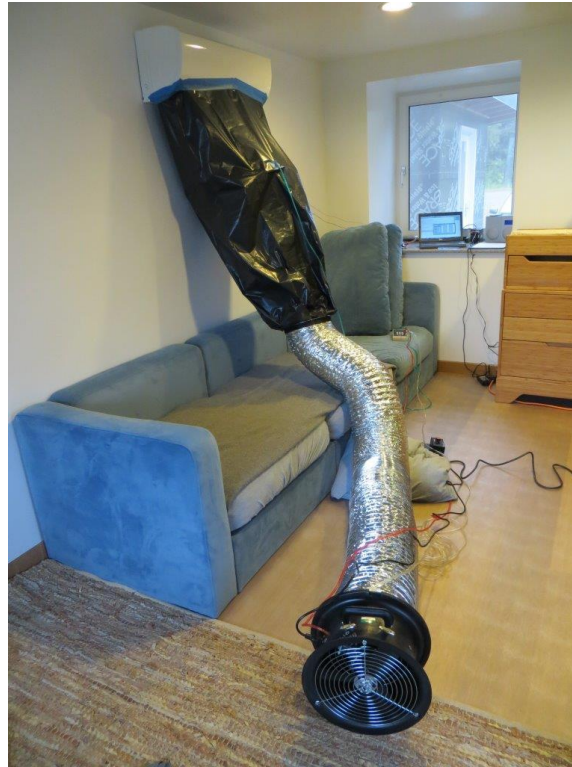
Figure 9: Duct blaster set-up for calibration of the anemometer.
